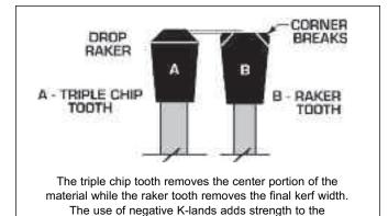
cutting edge and protects it from damage.
